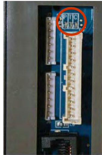
T7 EPP's three LEDs are P, T, C (left to right)
