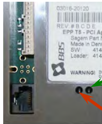
T5 EPP's two LEDs
